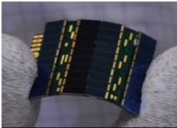
Fig. 4: Array of solar cells mounted on a flexible PCB to harvest energy from ambient light.
