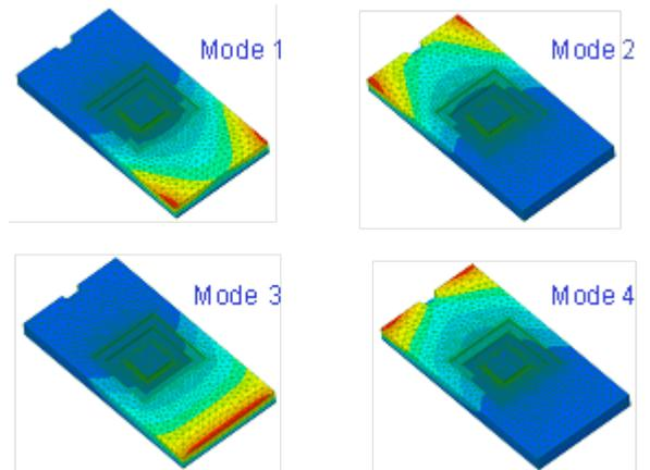
Figure 7 : Vibration modes of die attach without encapsulant.
