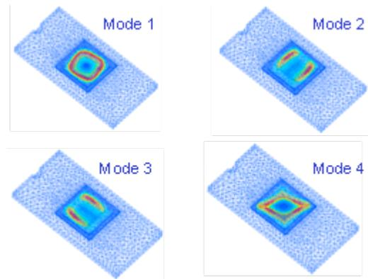
Figure 6 : Vibration modes of die attach with encapsulant.
